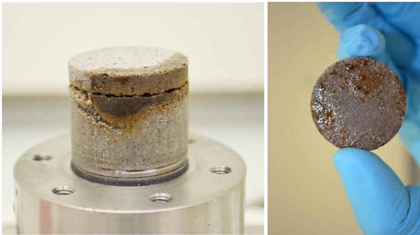
Figure 3-2 Image of compacted, water saturated and spiked MX-80 of test cell 15 after incubation (left) and the concrete plug surface which was in contact with the bentonite clay (right).
