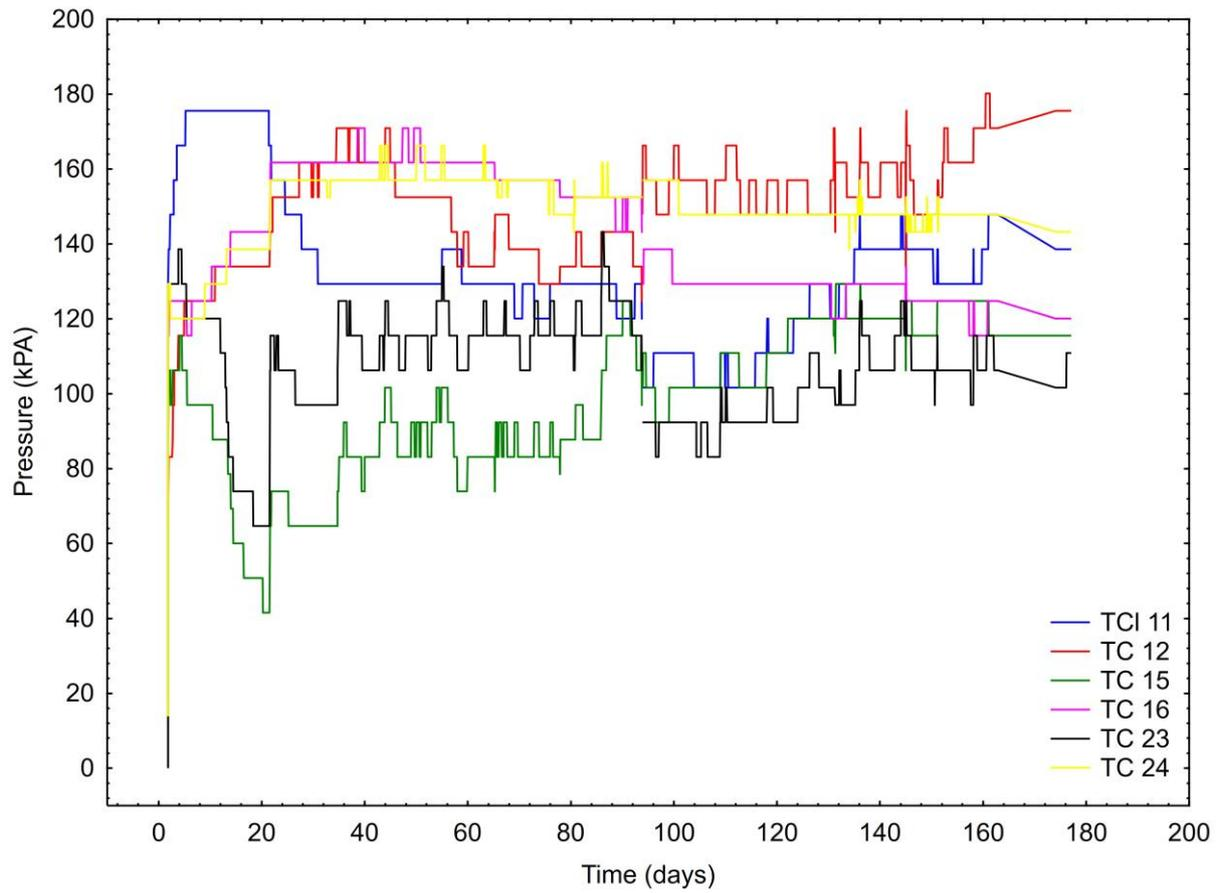
Figure 3-1 Pressures registered by force transducers over time, test cells according to symbol description.
