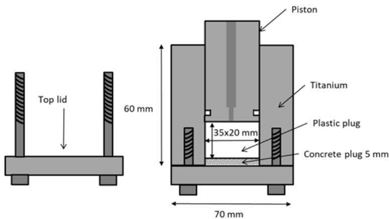
Figure 2-1 Scheme of a test cell with concrete- and plastic plug.
