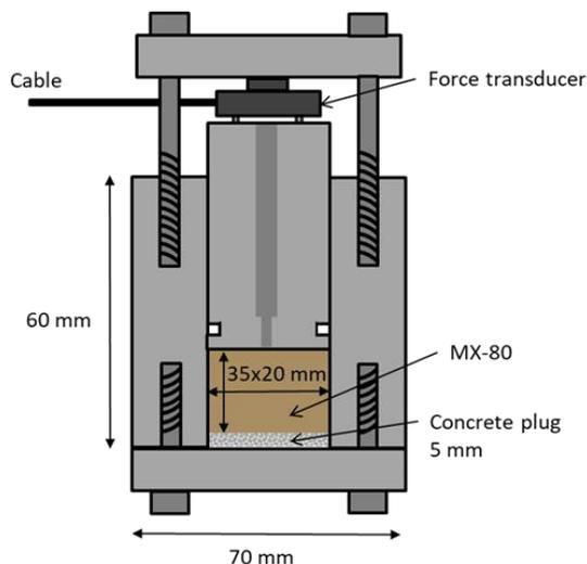
Figure 2-2 Scheme of an assembled test cell with MX-80 and concrete plug.
